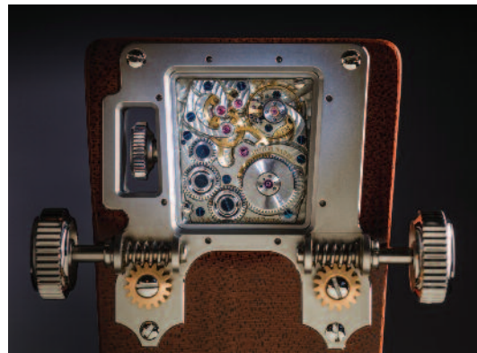
Attention to detail: Closeup of the RGM timepiece built into the headstock.
